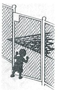
These are the gates people must walk through. Swimming pool barriers should be equipped with a gate or gates which restrict access to the pool. A locking device must be included in the gate design. Pedestrian gates must open outward and away from the pool and shall be self-closing and self-latching.
